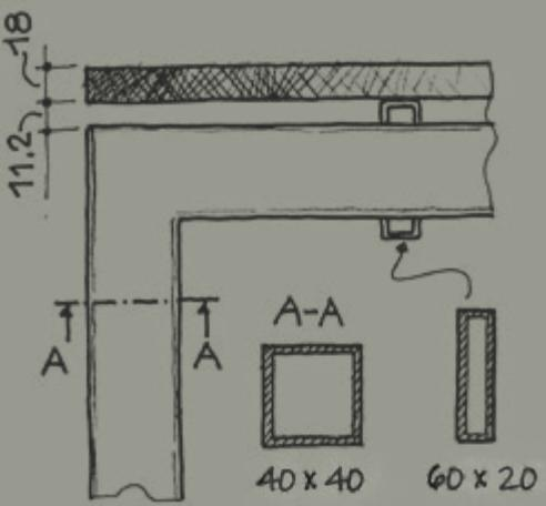
**Fixing** the worksurface is secured to the structure through conical pins which are inserted onto metal springs applied to the beams. The table top is installed only by pressure, without the use of screws. The horizontal beams also provide support to several accessories.
